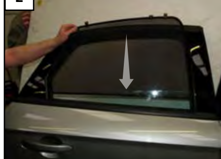
2 Install shade into side window
